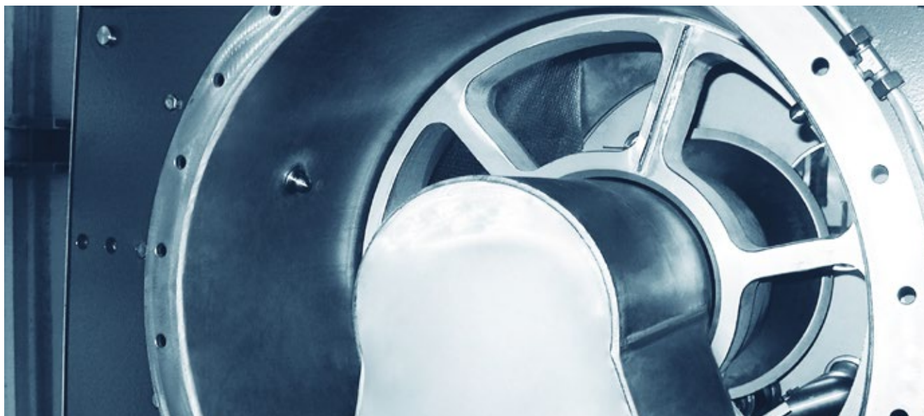
Solids discharge outlet
